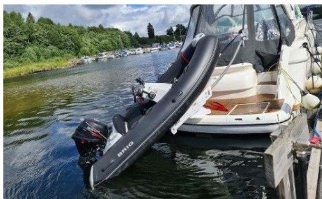
The tender is winched onto the cradle with the winch arm in the square tube.
