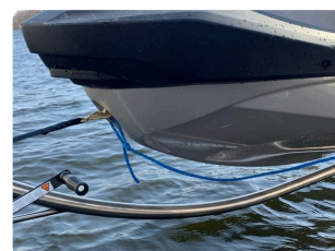
The curved arm gives a level pull on the hook.
