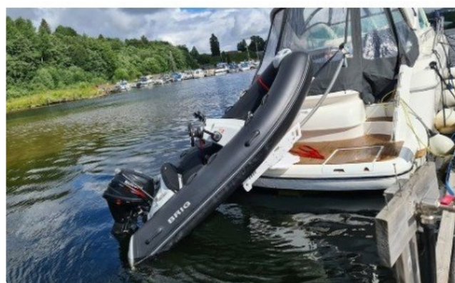
The tender is winched onto the cradle with the winch arm in the square tube.
